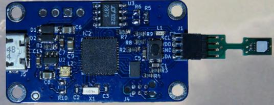
Airborne Innovations has introduced new technology to aid in icing avoidance and situational awareness. This experimental sensor is designed to help detect potential icing conditions before ice accumulation becomes a problem.
