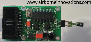
Airborne Innovations has introduced new technology to aid in icing avoidance and situational awareness. This experimental sensor is designed to help detect potential icing conditions before ice accumulation becomes a problem.
